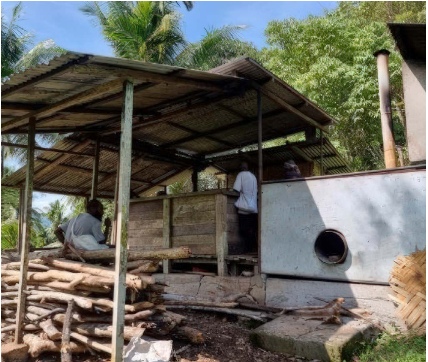
Traditional cocoa bean dryers require heavy labour and large amounts of timber for fuel. These wood-powered dryers also contribute to deforestation and carbon emissions.
