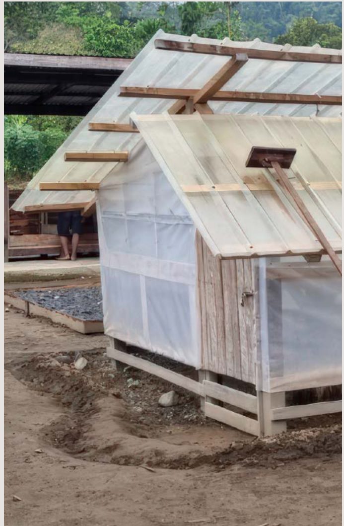
The Cocoa project is piloting the use of an environmentally friendly solar dryer. This is an innovative approach that can produce better quality dried beans.
