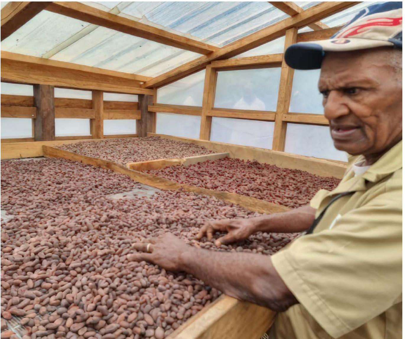
The Cocoa project's Technical Officer explains the drying process inside the greenhouse solar dryer.
